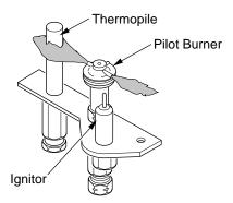
Figure 42 - Correct Pilot Flame Pattern
